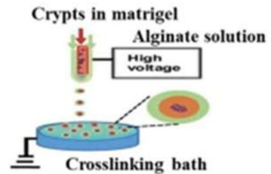
Schematic diagram of extrusion method - a two-fluidic electro-spraying method for encapsulation of cells in core-shell capsules.
